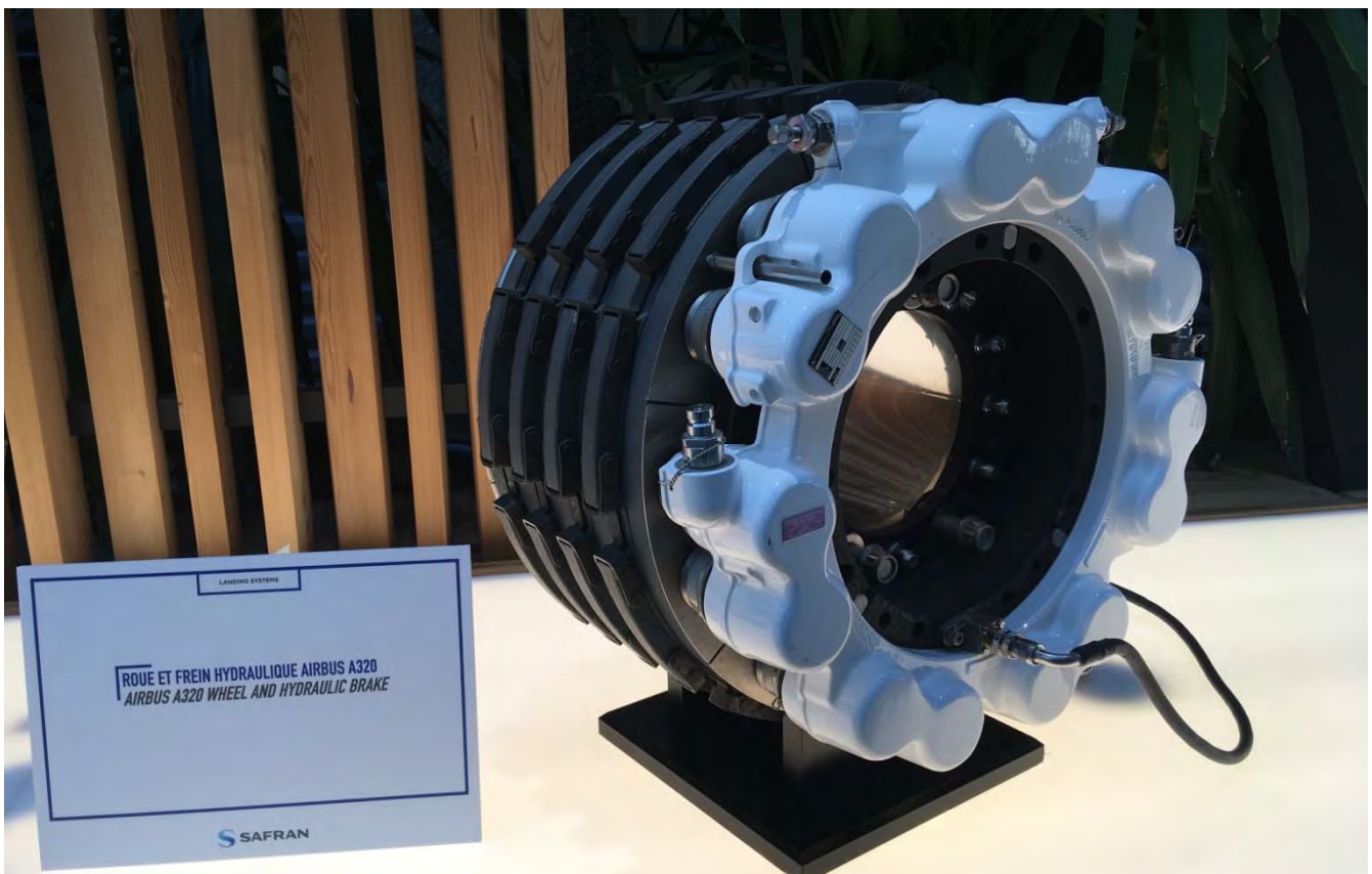
Frein carbone hydraulique Airbus A320 © Safran p.6
